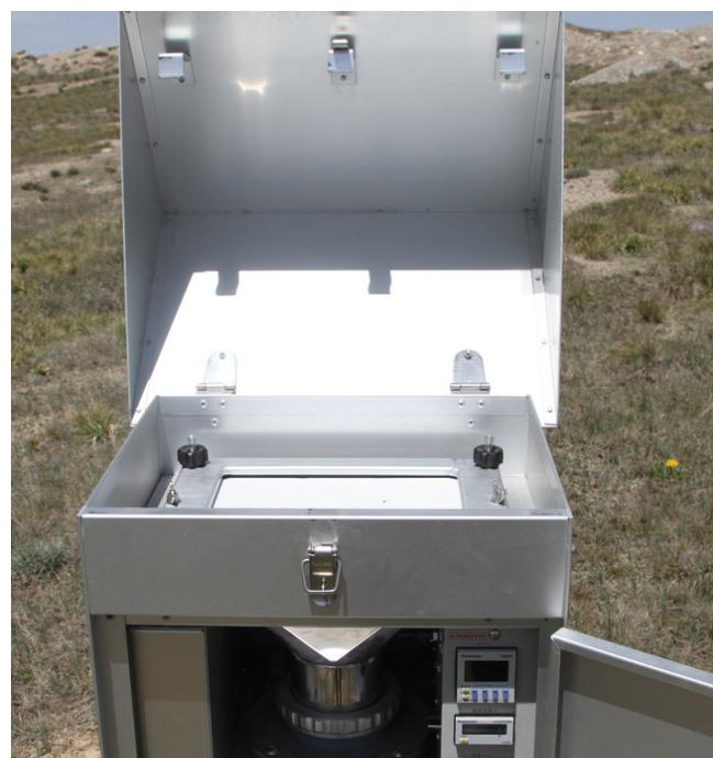
Figure 13: Dust sampler
