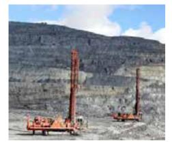
Drilling plays an essential role in extraction of precious metals. Before any major work can begin on a given section, geologists must have a precise idea of the average gold grade in the ore. Based on the drilling data they will then decide whether to process the ore at the mill, or haul it to a waste rock dump, if the gold content is too low to make a profit.
