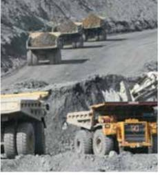
In order to get at the gold ore, large sections of rock that contain little or no gold also need to be removed. This was 'waste rock' is hauled to designated waste rock dumps and unloaded there. Trucks transporting gold ore on the other hand go to the mill. Here the ore is ground down to a fine powder and is transported to the factory by a conveyor belt
