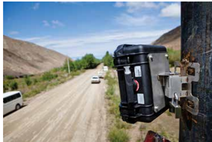
Vehicle counter device logs direction and size of vehicles traveling on the technical road.
