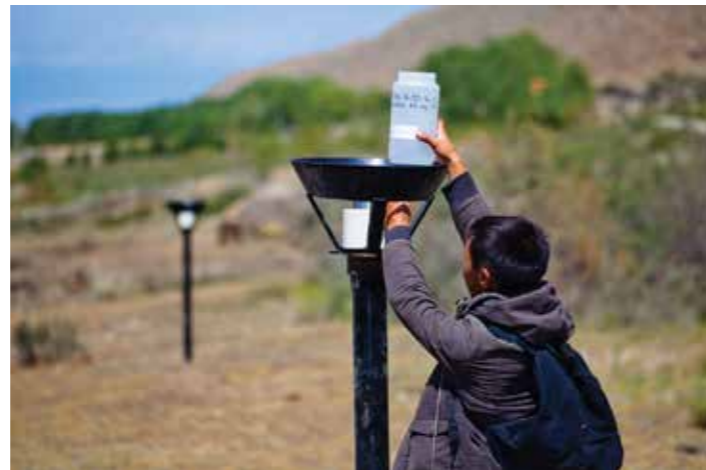
Jashyl-Oi eco-camp participant installing a dust trap.
