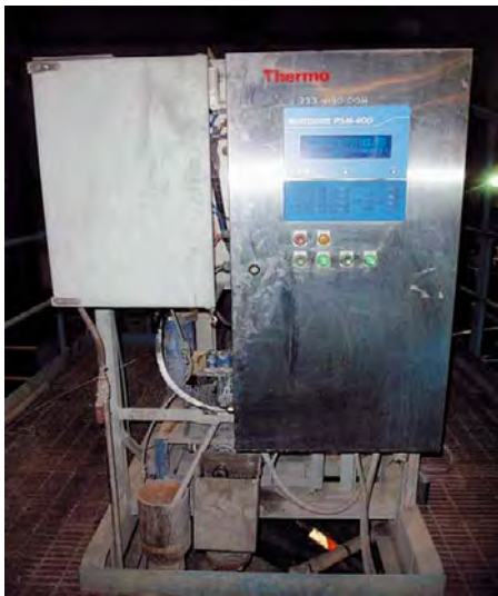
Photo 2-3: Thermo Multipoint PSM 400 analyzer
